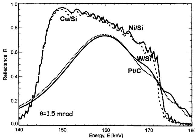
**Figure 7.** Theoretical reflectance curves for Ni/Si (long dashed), Cu/Si (dashed), W/Si (solid) and Pt/C (dotted) depth-graded multilayers containing 600 bilayers, optimized for use over the energy range from  $145 < E < 175$  keV.
