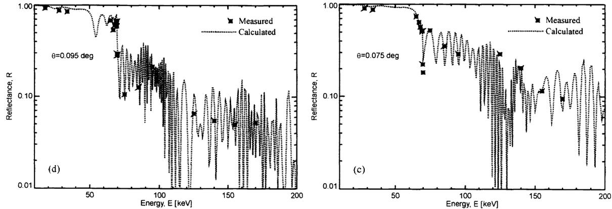
**Figure 5.** Reflectance vs. energy data for a depth-graded W/Si multilayer, identical to the one shown in Fig. 4, measured at  $\theta=0.095^\circ$  (a) and  $\theta=0.075^\circ$  (b). Shown for comparison are calculations made using a depth-graded distribution of interface widths in the range  $\sigma=0.275 - 0.35$  nm.
