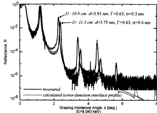
**Figure 2.** Specular X-ray ( $E=8.04$  keV) reflectance for periodic W/Si multilayers containing 100 bilayers, deposited at  $P_{Ar}=2$  mTorr, and with target-to-substrate distances  $D=10.8$  cm and  $D=11.5$  cm.
