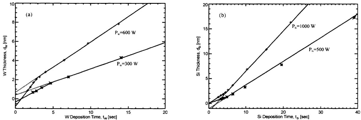
**Figure 3.** Layer thickness vs. deposition time for W (a) and Si (b) determined from X-ray reflectance analysis of multilayer films deposited at the magnetron powers indicated. Also shown are bi-linear fits to these data.
