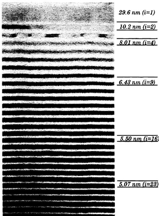
**Figure 4.** Cross-sectional transmission electron micrograph of the top portion (i.e., the top ~28 bilayers) of a depth-graded W/Si multilayer structure. Selected bilayer indices and thicknesses are indicated. The W (dark bands) and Si (light bands) layers are separated by thin amorphous W-Si interlayers (grey bands). Note that the topmost Si layer is not completely visible in this image.
