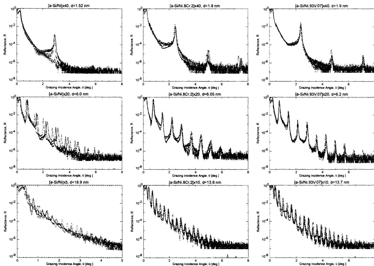
**Figure 8.** X-ray reflectance measured for periodic Ni/Si,  $\text{Ni}_8\text{Cr}_2/\text{Si}$  and  $\text{Ni}_{93}\text{V}_{07}/\text{Si}$  multilayers. Curves are shown for as-deposited (solid) samples, as well as samples measured after 1-hour thermal anneal in air at 100°C (dotted), 200°C (dashed) and 300°C (dot-dashed). The number of bilayers are indicated, as are the multilayer periods (d) determined for the as-deposited samples.
