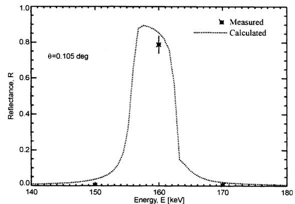
**Figure 6.** Measured reflectance vs. energy at  $\theta=0.105^\circ$  for a W/Si multilayer containing 800 bilayers, with bilayer thicknesses in the range  $2.09 < d < 2.25$  nm. The calculated reflectance using  $\sigma=0.3$  nm interface widths is shown for comparison.
