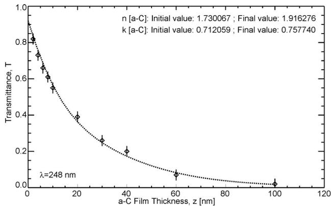
FIG. 1. Measured transmittance (diamonds) of *a*-C films deposited onto quartz substrates at a photon wavelength of  $\lambda=248$  nm. The calculated transmittance (dotted line) is also shown, and is computed from the best-fit values of the optical constants ( $n$ ,  $k$ ) as indicated.
