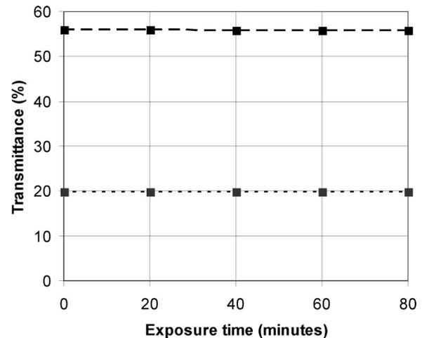
FIG. 2. Measured transmittance for two  $a$ -C films as a function of time after exposure to high-intensity 248 nm radiation as described in the text.
