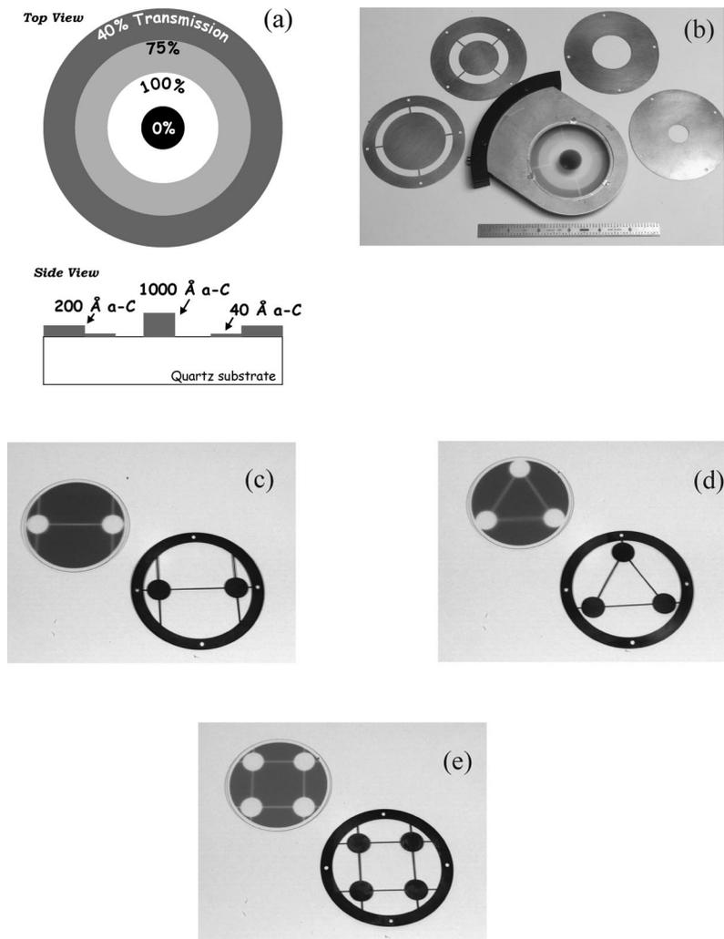
FIG. 3. Schematic diagram of (a) a concentric-ring-type variable-transmission aperture. A photograph of the actual aperture is shown in (b), along with the stencil masks used during fabrication, described in the text. (c) Dipole, (d) tripole, and (e) quadrupole apertures are also shown, along with the stencil masks used for fabrication.
